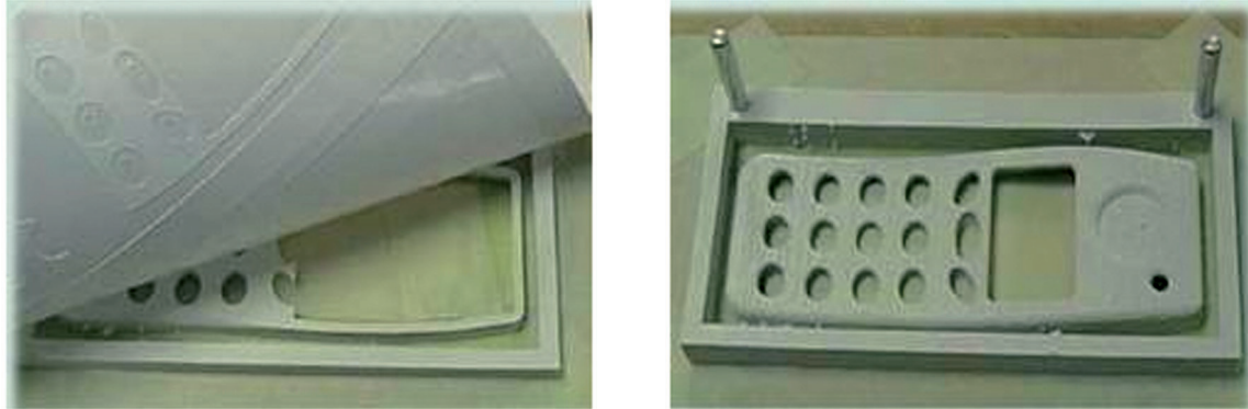
Figure C3: Laminated object manufacture using Boxford's RapidPro
